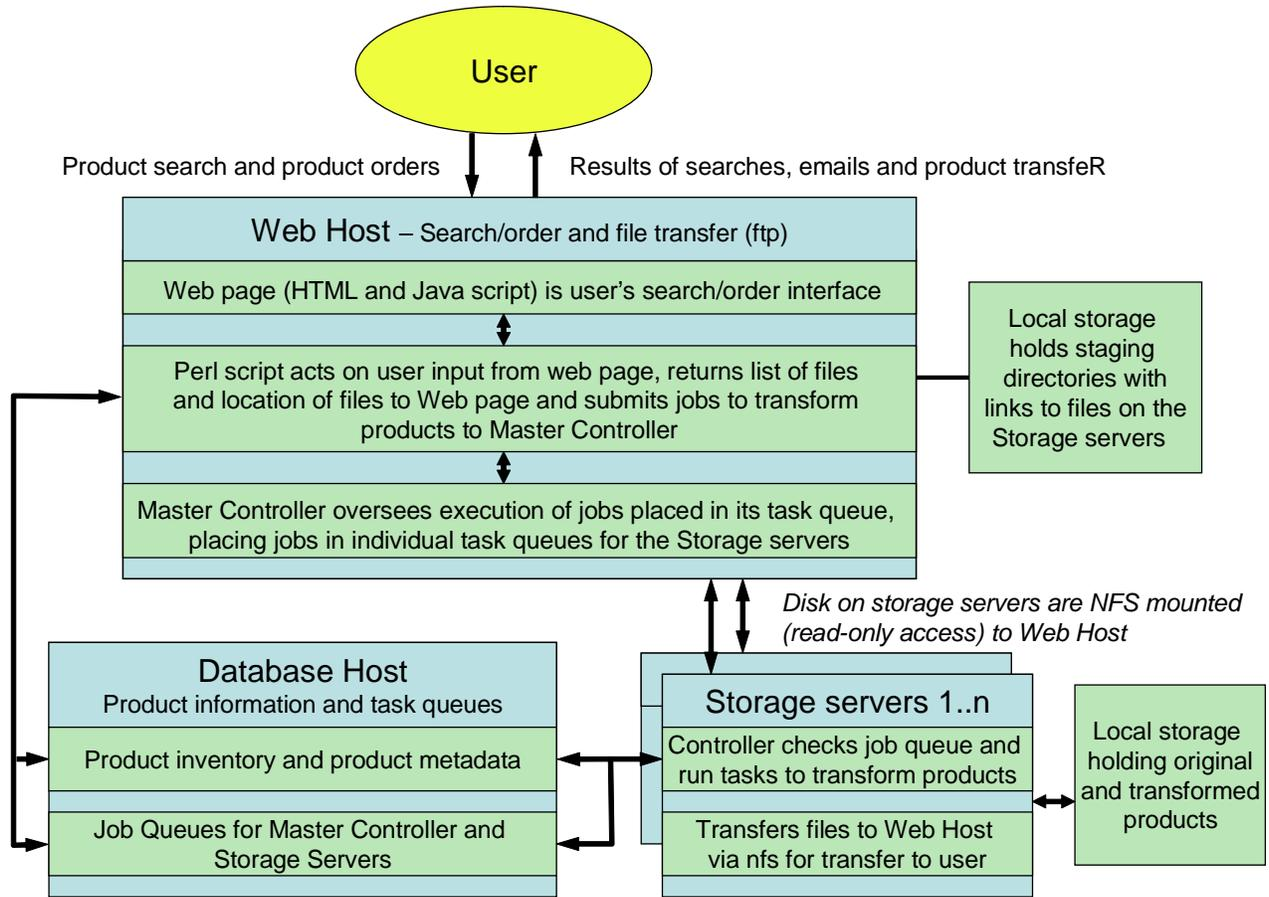
**Figure 4.** Architecture of the product distribution system.
