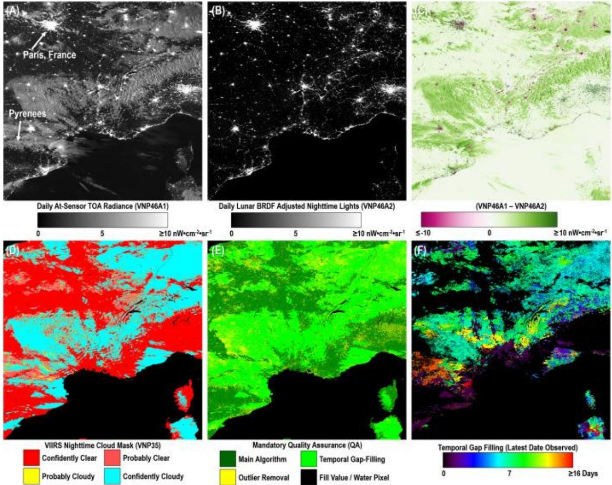
**Figure 4** Black Marble product suite components for a  $10^\circ \times 10^\circ$  Level 3 tile over France and the Balearic Sea region (h18v04; DOY 2015-091). The full-moon-illuminated and 51% cloud-contaminated scene illustrates the challenges of nighttime cloud masking over snow-covered surfaces (e.g., the French Alps and the Pyrenees).
