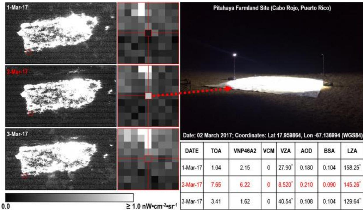
**Figure 7** The NTL radiance at the Pitahaya farmland site in Cabo Rojo, PR on 1st, 2nd and 3rd March 2017. The top-right image shows the setup of the stable point source. TOA and VNP46A2 values are in  $\text{nW} \cdot \text{cm}^{-2} \cdot \text{sr}^{-1}$ . VCM = 0 represents cloud free overpasses. LZA is lunar zenith angle, and the values larger than  $108^\circ$  correspond to moonless nights.
